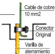
**Cable a tierra (cobre)** \_\_\_\_\_
